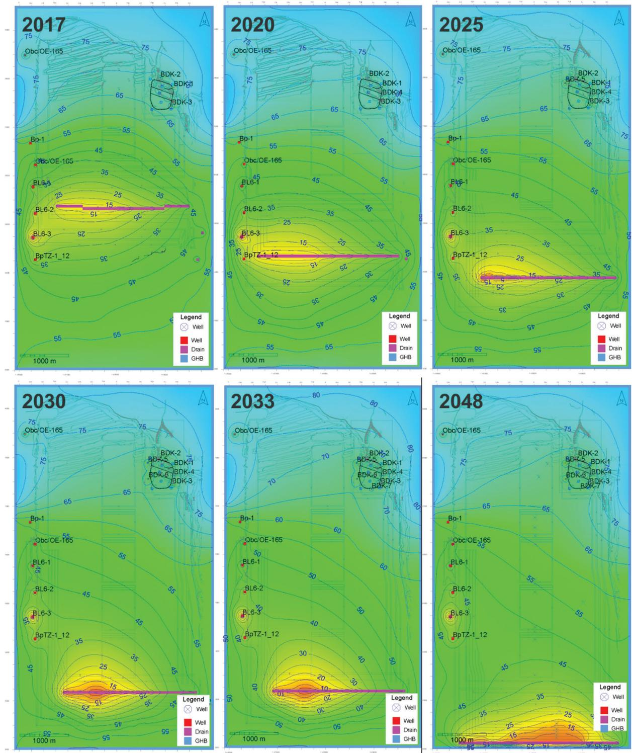
Fig. 1. Predictive hydrodynamic calculations – the piezometric levels for the future period (2017–2048)
