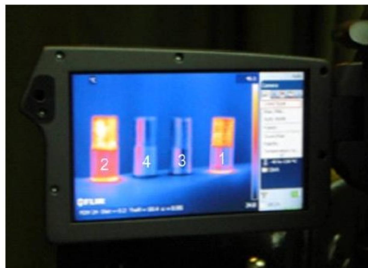
Fig. 10. Photograph of thermal camera display of thermal image during testing of the effect of cadmium plating on the temperature distributions of the threads
