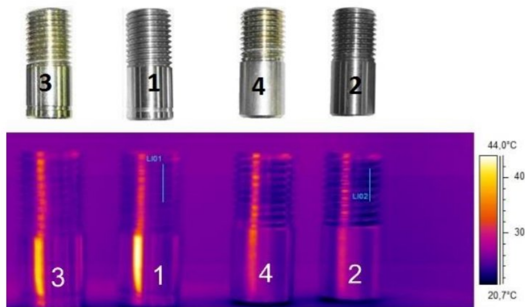
Fig. 6. Photograph and thermal images of threaded fastenings, type M 33 × 2: 1 and 2 have cut and cold-rolled threads with no cadmium finish, and 3 and 4 have cut and cold-rolled threads with cadmium finish.
