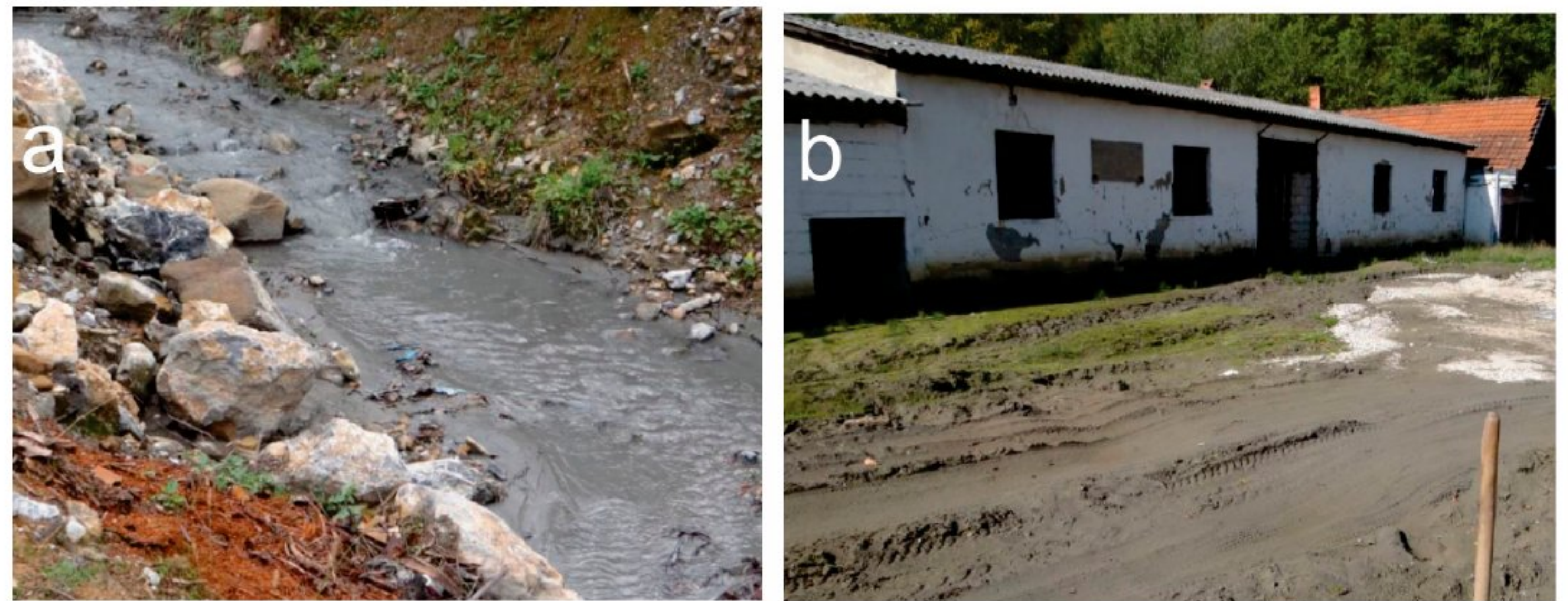
Figure 8. Tailings deposits in the bed of the Kostajnička River (a) and on the surrounding terrain (b). Reproduced with permission from the Water Institute “Jaroslav Černi” [10].
