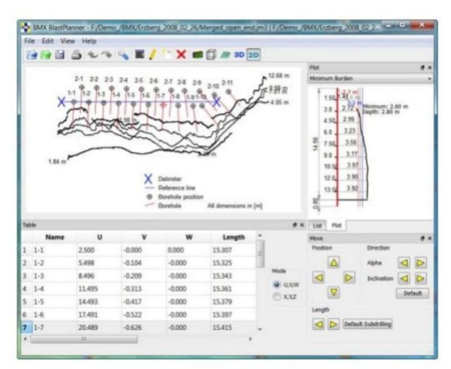
**Figure 3** Software framework displaying drilling parameters and the profile of the borehole (3gsm gmbh, 2019)
