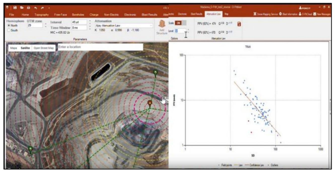
Figure 7 Analysis of seismic effect and diagram of allowed PPV (O-pitblast, 2019)
