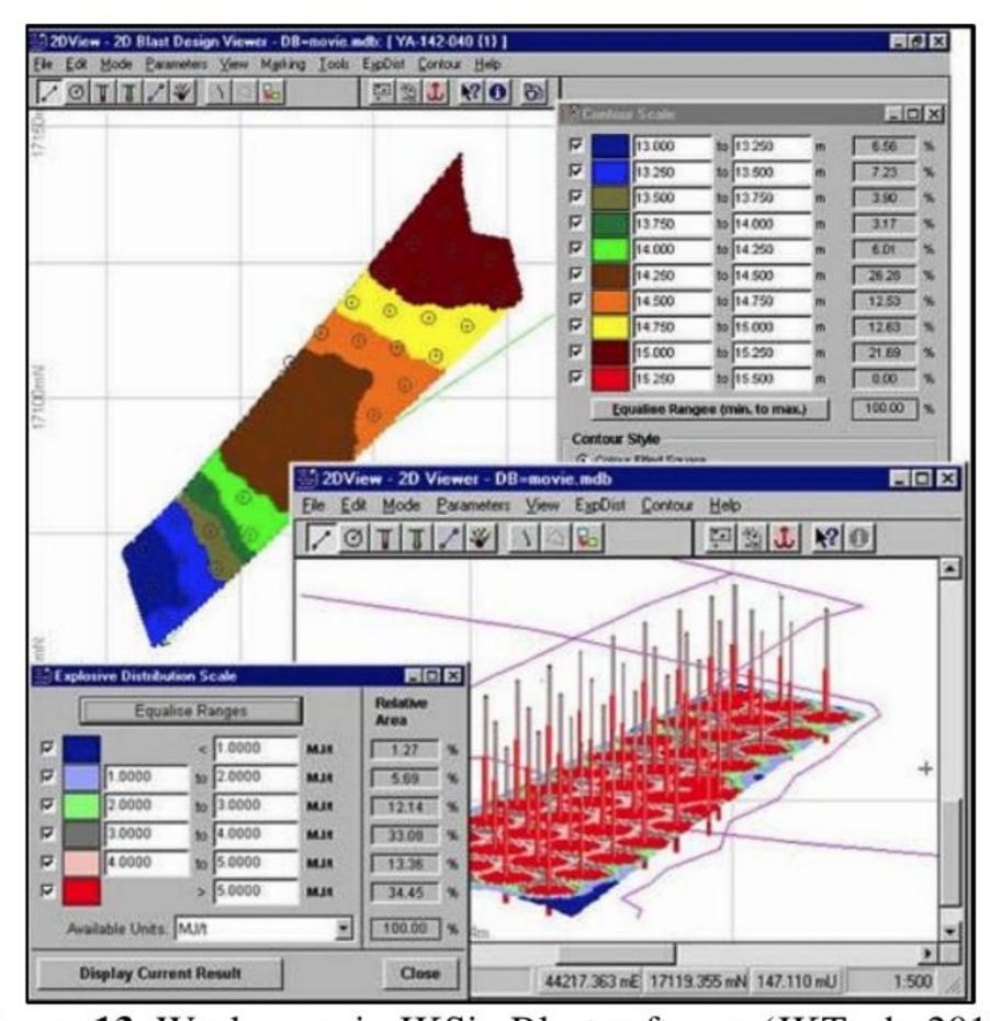
Figure 13 Workspace in JKSimBlast software (JKTech, 2019).
