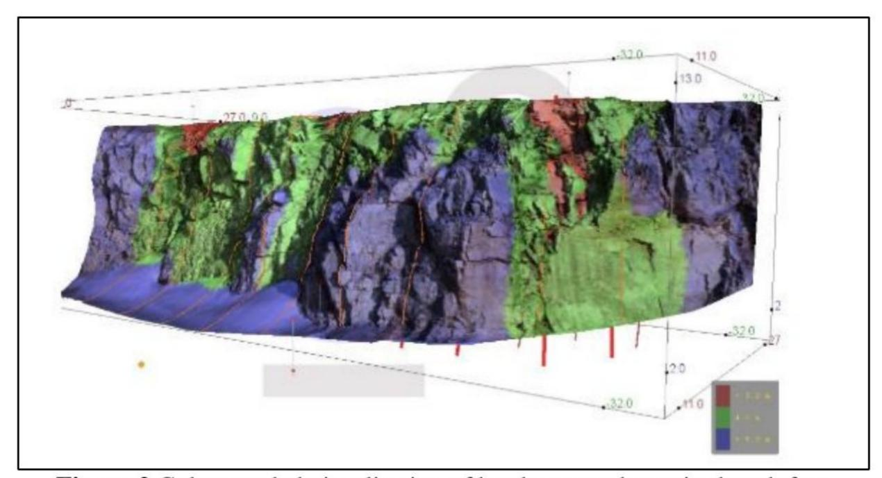
Figure 2 Colour-coded visualisation of burden over the entire bench face (3gsm gmbh, 2019)
