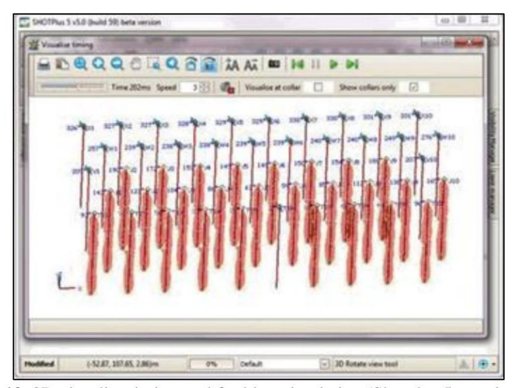
**Figure 10** 3D visualise timing tool for blast simulation (Shotplus 5 premier, 2019).
