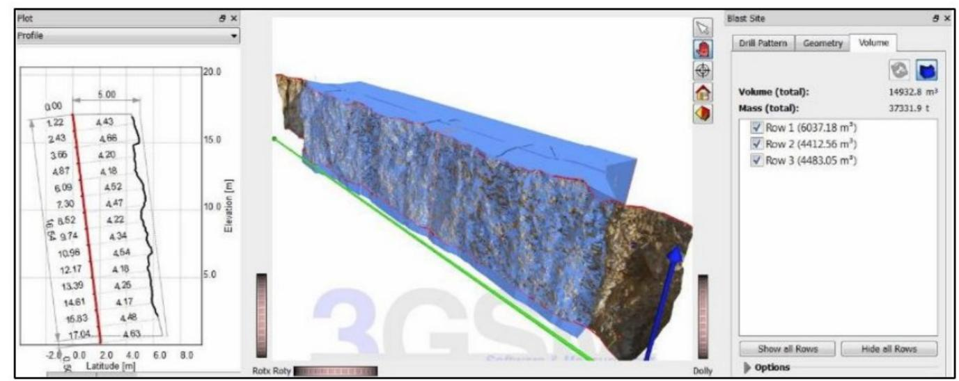
**Figure 4** Bench model for calculating the volume of fragmented rock material (3gsm gmbh, 2019)
