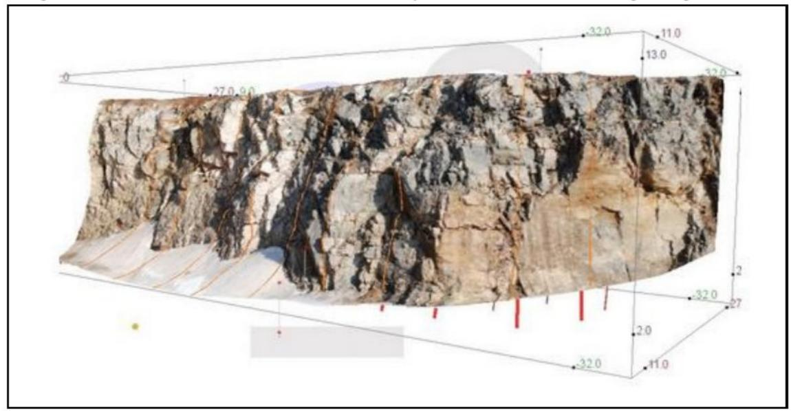
Figure 1 3D image of a bench face with planned boreholes and visualised profiles (3gsm gmbh, 2019)
