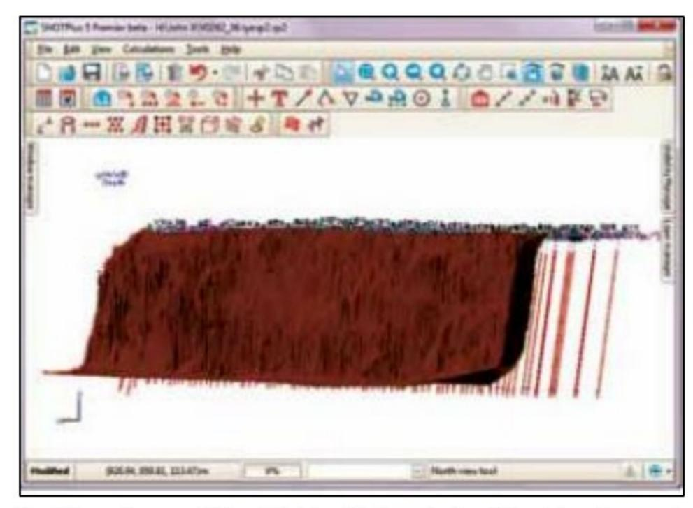
Figure 11 3D surfaces of blast field with boreholes (Shotplus 5 premier, 2019)
