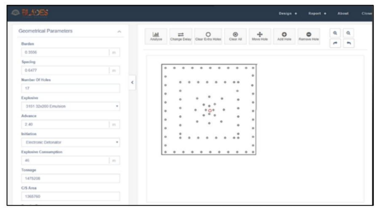
Figure 9 Blast design in underground excavation by Tunnel Designer Software (Mineexcellence, 2019)
