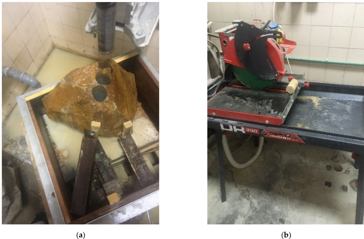
Figure 3. Procedure for preparation of specimen for laboratory tests: (a) drilling process, (b) cutting process.
