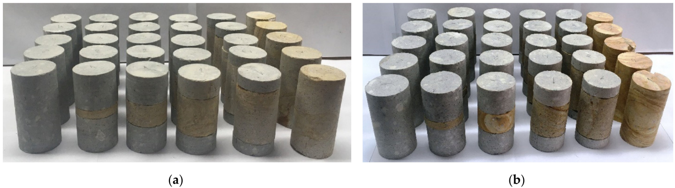
Figure 5. Composite specimens prepared for testing: (a) UCS, and (b) triaxial test.
