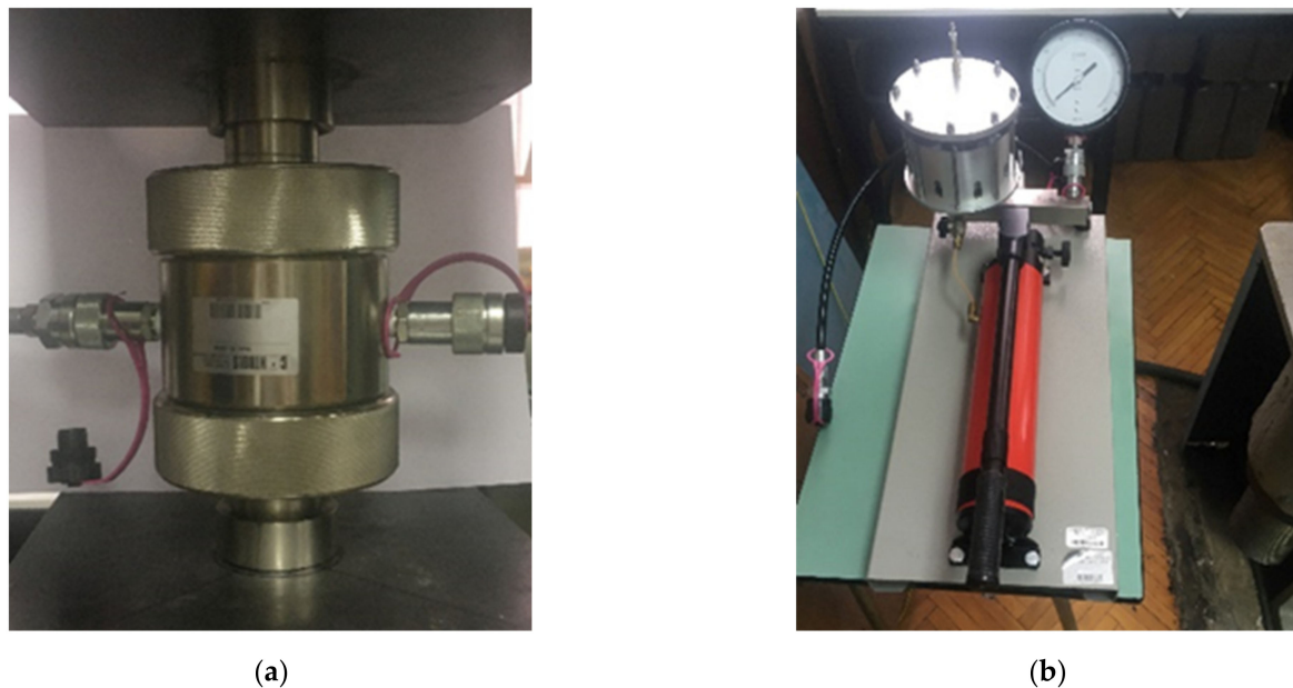
Figure 6. Triaxial test equipment: (a) Hoek cell and (b) manual confining pressure system for testing.
