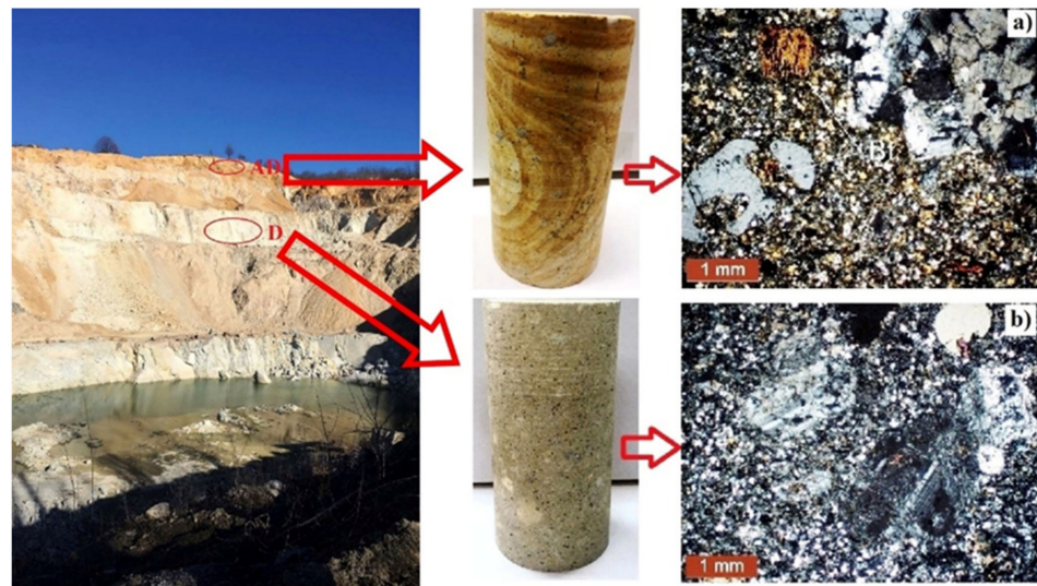
Figure 2. Analyzed open pit slope consisting of dacite with microscopic images of the material: (a) altered dacite and (b) dacite.
