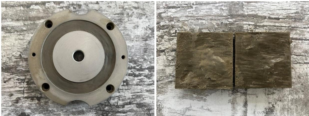
Figure 5. Appearance of the gray clay samples after testing in the ring shear apparatus (left) and direct shear apparatus (right).
