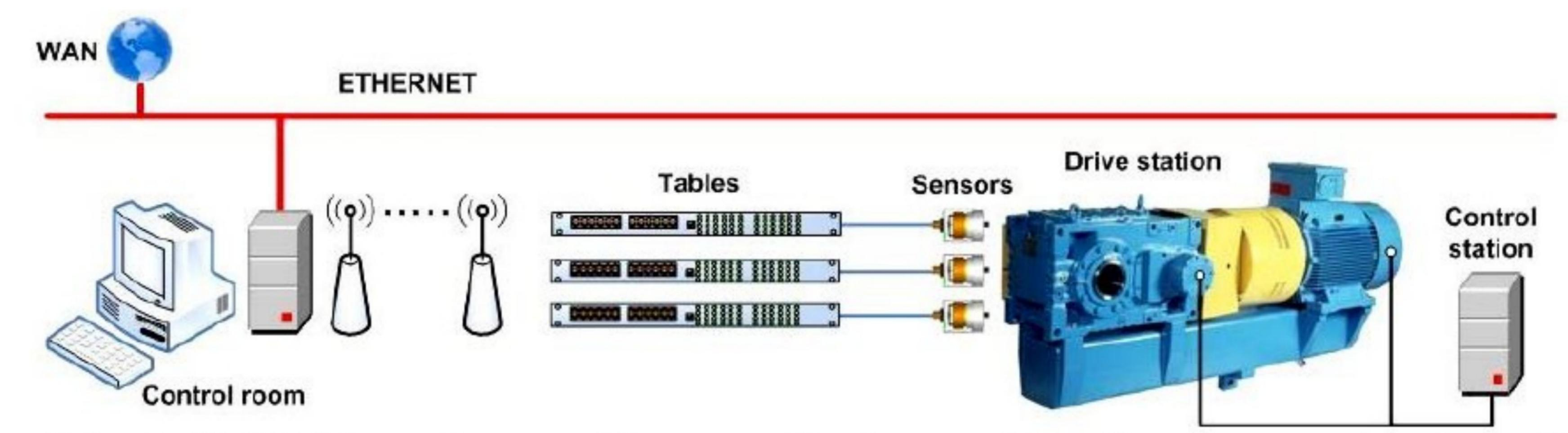
Fig. 4 Definition of proactive monitoring system for gear-reduction of belt conveyor drive (tele-diagnostics)
