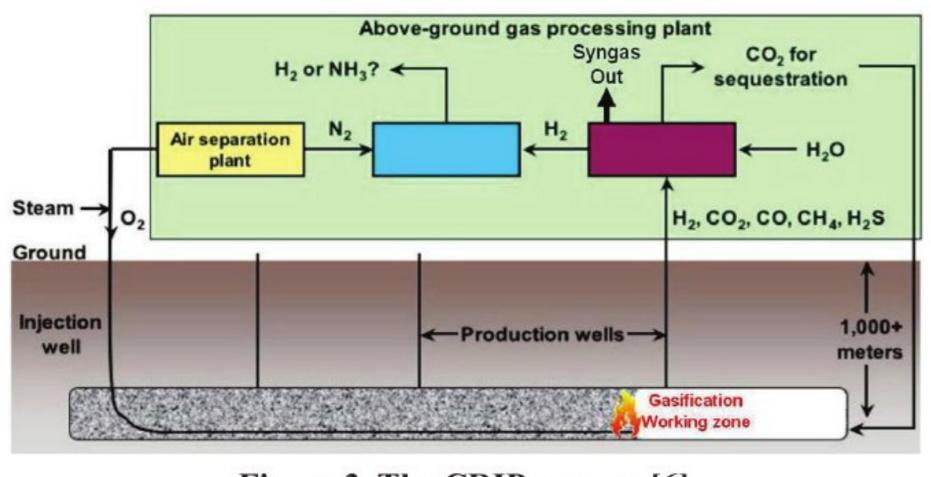
The injection boreholes are drilled vertically through a semicircular rounded layer prior to entering the part of the coal layer and continues horizontally to the production wells which are necessarily vertical [6]. When horizontal connections are established, the ignition starts at the end of the injection. At the end of the treatment of this reaction zone, the reaction cavity-zone is
