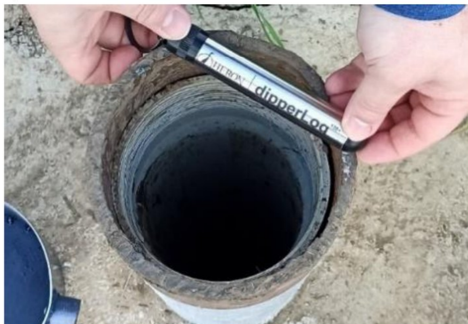
dipperLog 128+ sa opsegom merenja do 60 m dipperLog 128+ with a range of 60 m
