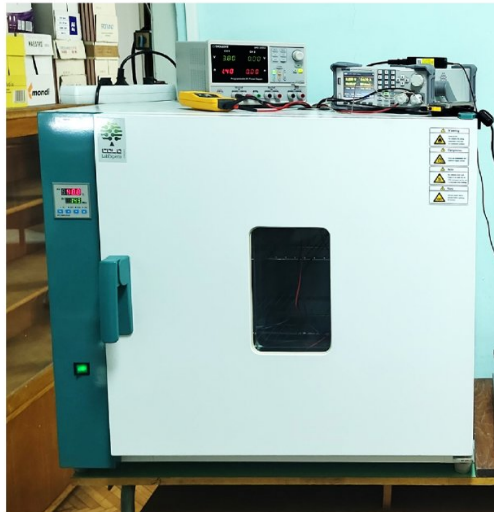
Fig. 1. Experiment setup (thermal chamber, electric load, power supply and voltmeter).
