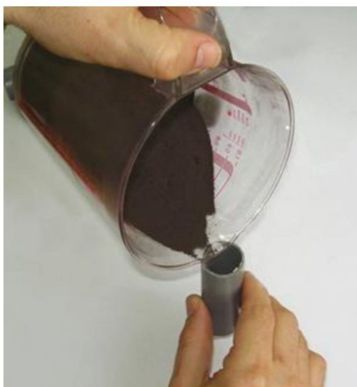
Fig. 1 Charging the cartridges with non-detonating chemical mixture [2,6]
