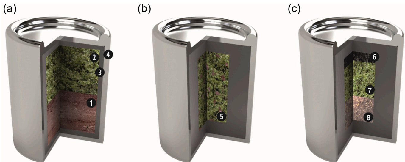
Fig. 3. The capsule with a schematic illustrations of three types of experimental setup used in reaction experiments. a) Layered setup comprising of sediment or metasome + peridotite. Noble metal capsule is loaded with layers of which the one lithology of choice (metasome, sediment or basaltic glass (1)) is placed in the bottom, and a layer of either lherzolite or harzburgite (2) is placed above; b) Mixed sediment + peridotite (5). In this setup, the two lithologies are intimately mixed; c) flow-through setup, which resemble the layered one with the addition of a melt trap. (3)- a graphite inner capsule; (4)- a noble metal outer capsule; (6)- a vitreous carbon melt trap; (7)- peridotite, and (8)- alkaline melt (glass).
