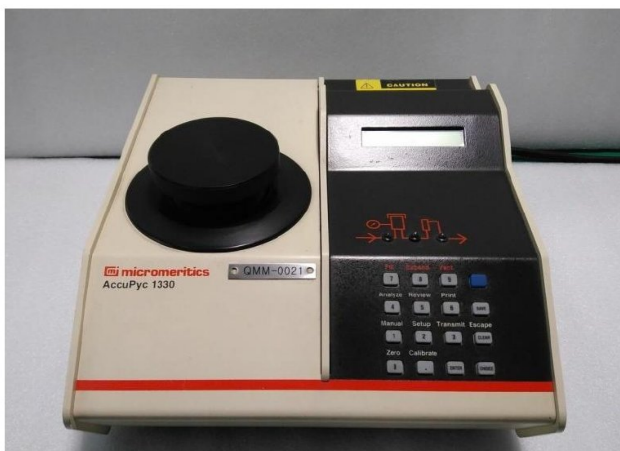
Slika 5.1: Automatizovani piknometar AccuPyc 1330 ( www.spwindustrial.com )
