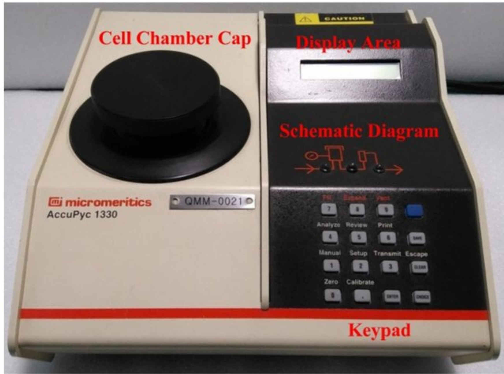
Fig. 8. Automated pycnometer AccuPyc 1330.
