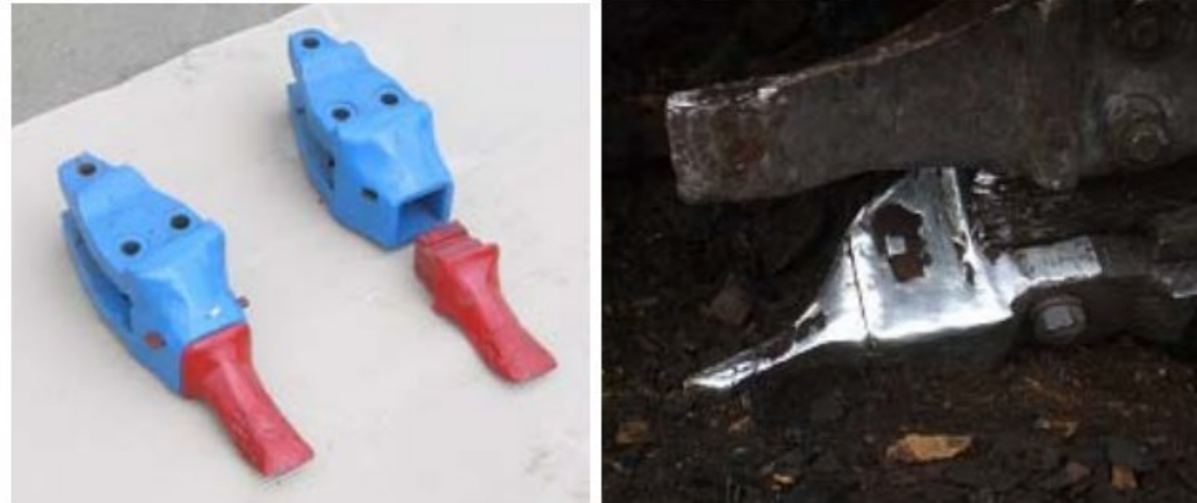
Fig. 21 Prototype and worn-out two-parted tooth for bucket chain excavator ERs 1000/20
