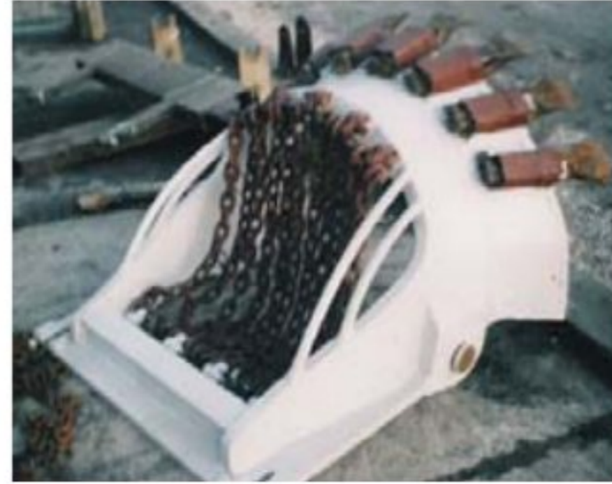
Fig. 15 Prototype of bucket with 4 supports for bucket wheel excavator SchRs 630
