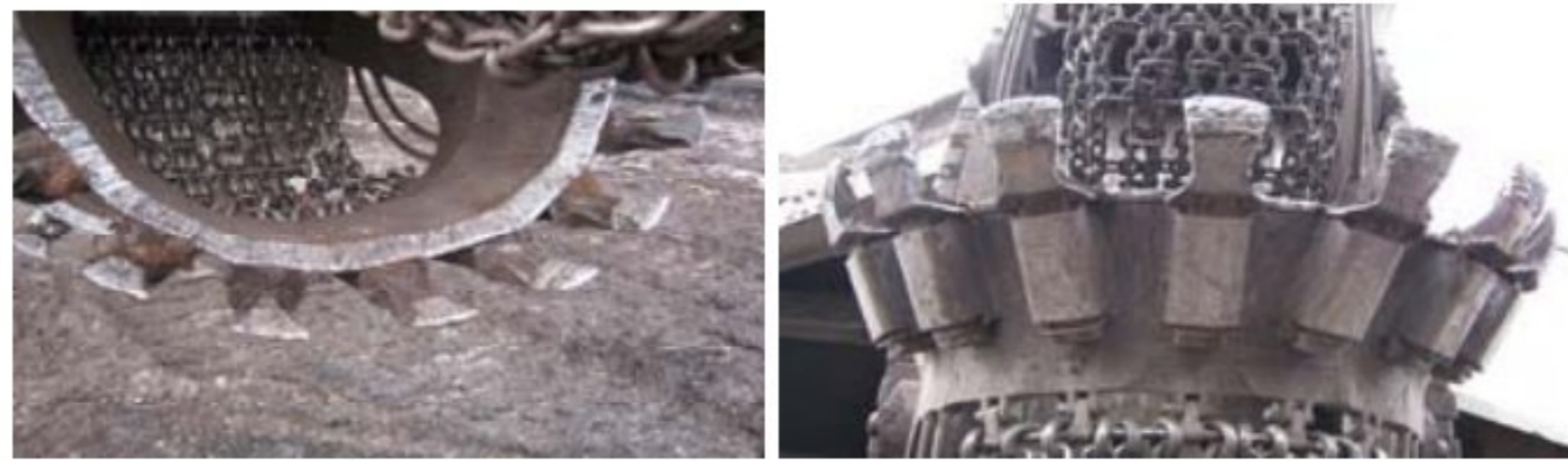
Fig. 6 Bucket with armoured teeth (welded)
