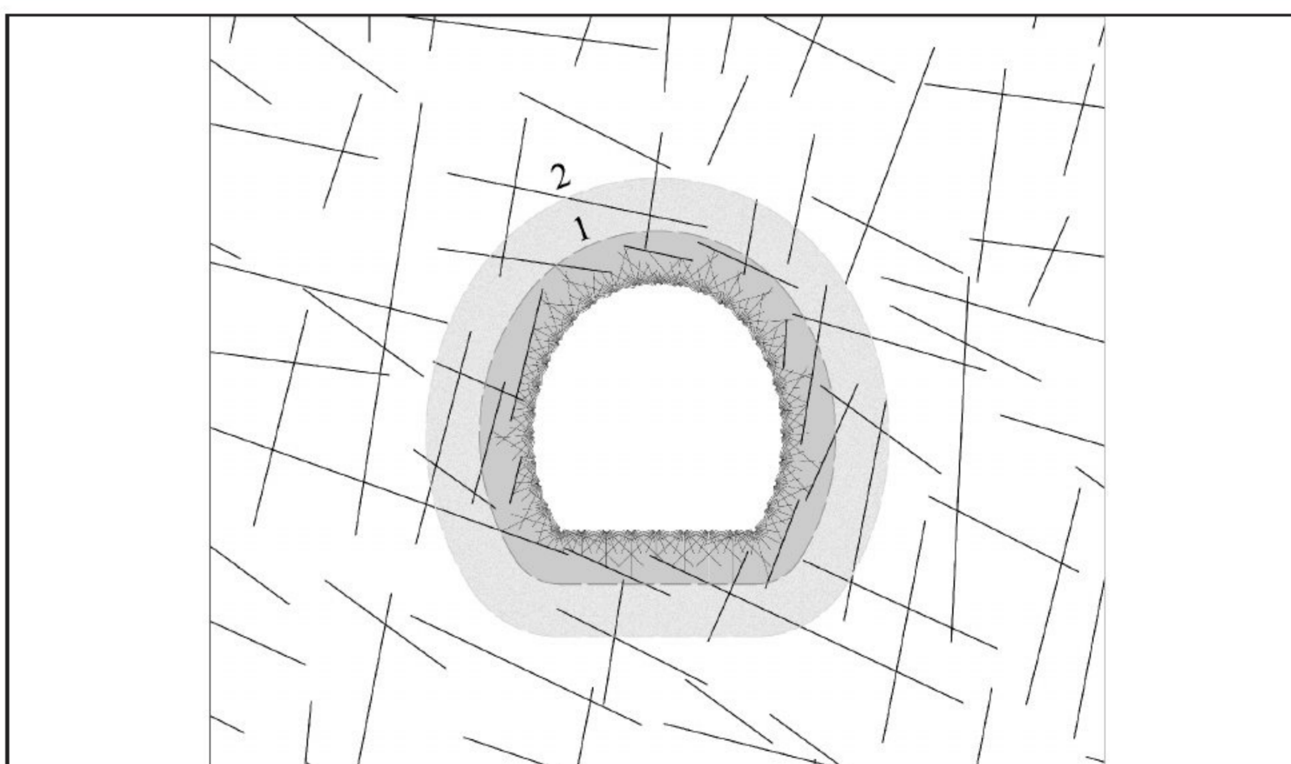
Figure 5 Blasting in rock mass where primary block sizes are smaller than the maximum length of the blast-induced radial cracks. Line 1 marks maximum length from contour blastholes to preexisting rock joints. Line 2 marks maximum length of blast induced radial cracks in monolith block. As can be seen, preexisting joints in rock mass are limiting radial crack propagation and therefore the blast damaged zone around the excavation has a smaller extent.
