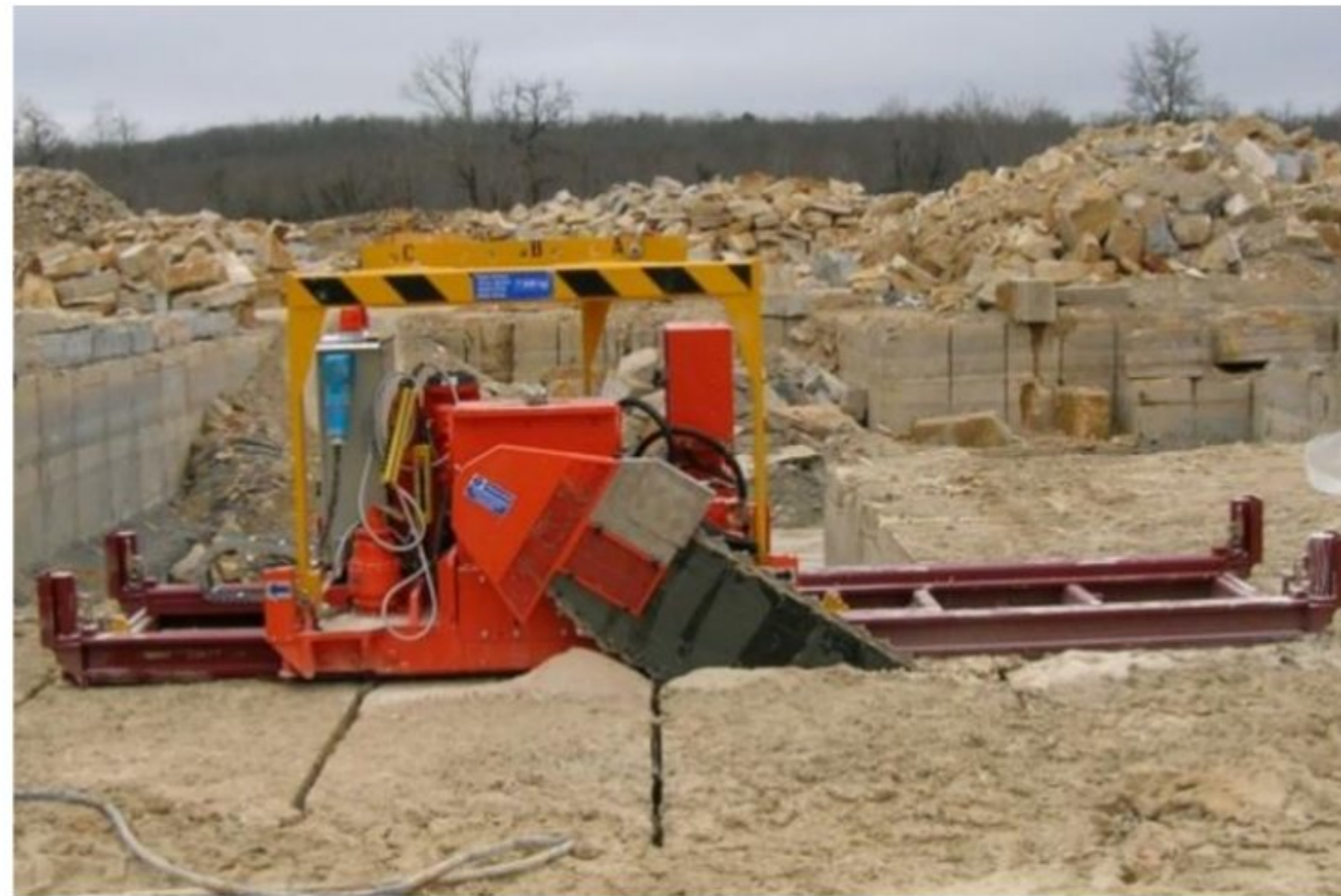
Figure 9 Chain saw machine by Italian company FANTINI (Fantini, 2023)
