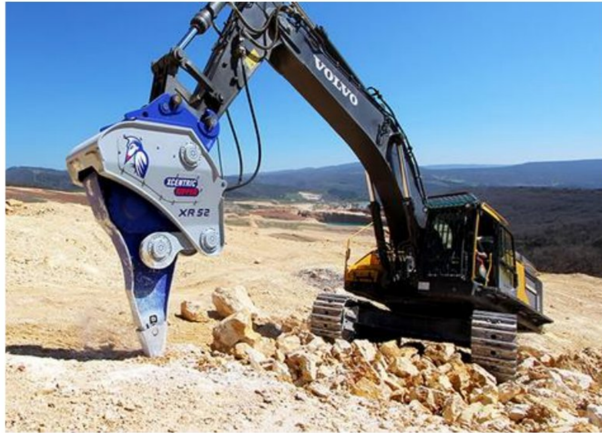
Figure 14 Hydraulic excavator with the ripper (Xcentric, 2023)
