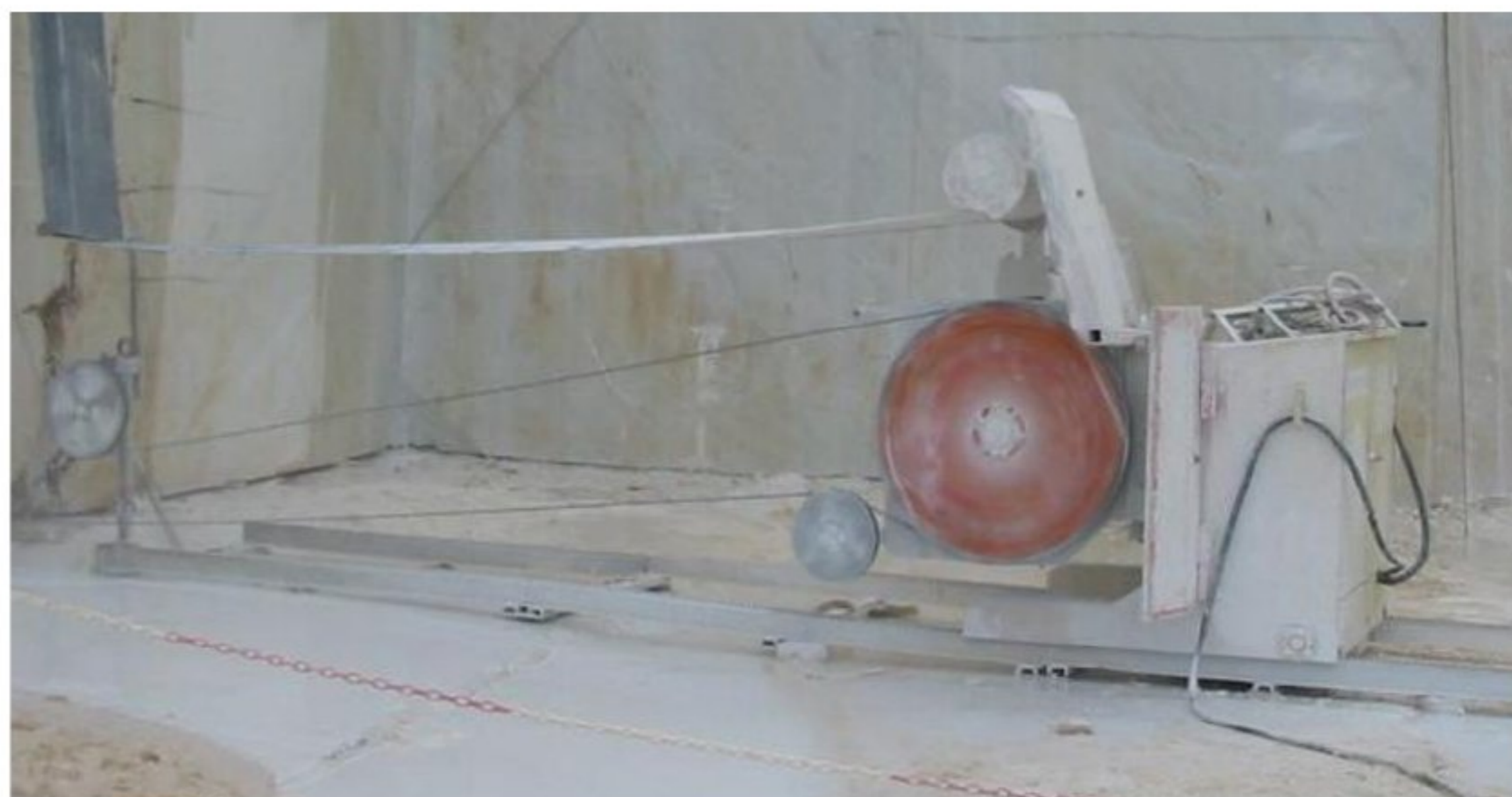
Figure 11 Diamond wire saw machine by Italian company LOCHTMANS (Lochtmans, 2023)
